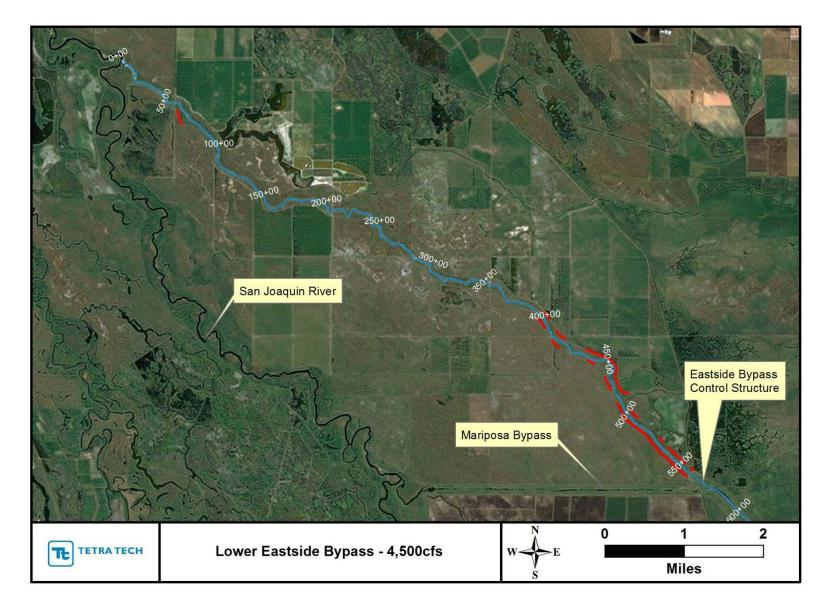
Figure 31. Portions of levee in the Lower Eastside Bypass where the 4,500-cfs water-surface elevation is above the existing outside ground elevation.
