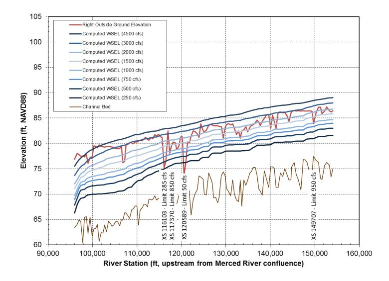
Figure 17. Comparison of outside ground elevation with computed water-surface elevations along right levee in Reach 4B2.
