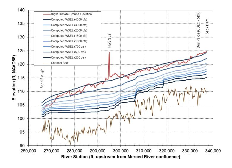
Figure 13. Comparison of outside ground elevation with computed water-surface elevations along right levee in Reach 4A.
