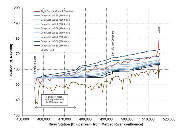
Figure 6. Comparison of outside ground elevation with computed water-surface elevations along right levee in Reach 2B.
