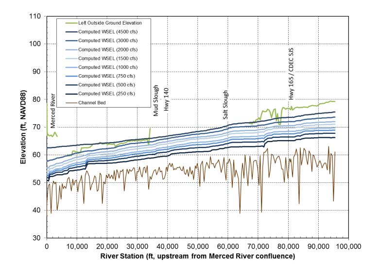
Figure 22. Comparison of outside ground elevation with computed water-surface elevations along left levee in Reach 5.
