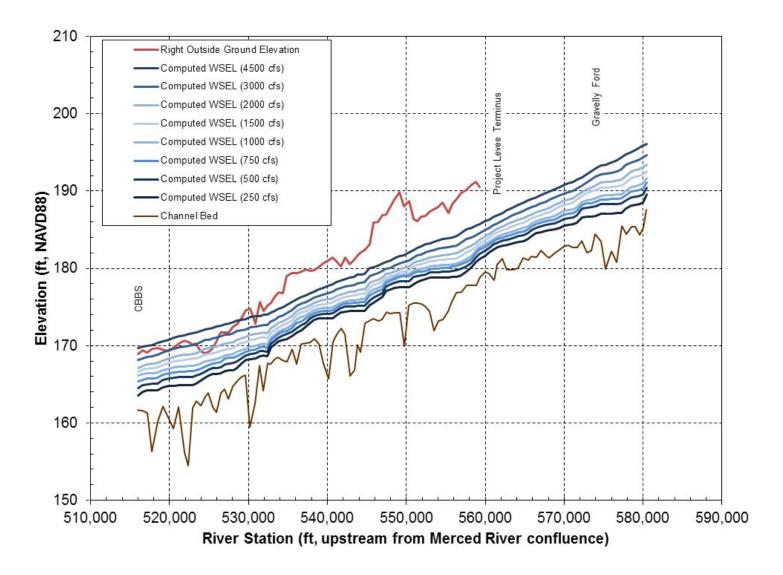
Figure 2. Comparison of outside ground profile with computed water-surface elevations along right levee in Reach 2A.
