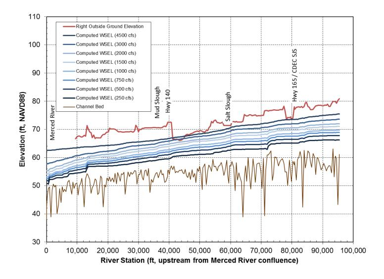
Figure 21. Comparison of outside ground elevation with computed water-surface elevations along right levee in Reach 5.
