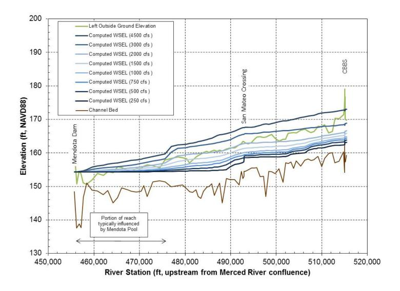
Figure 7. Comparison of outside ground elevation with computed water-surface elevations along left levee in Reach 2B.
